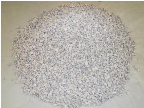
Fig. 3. Graduated recycled coarse aggregate.
