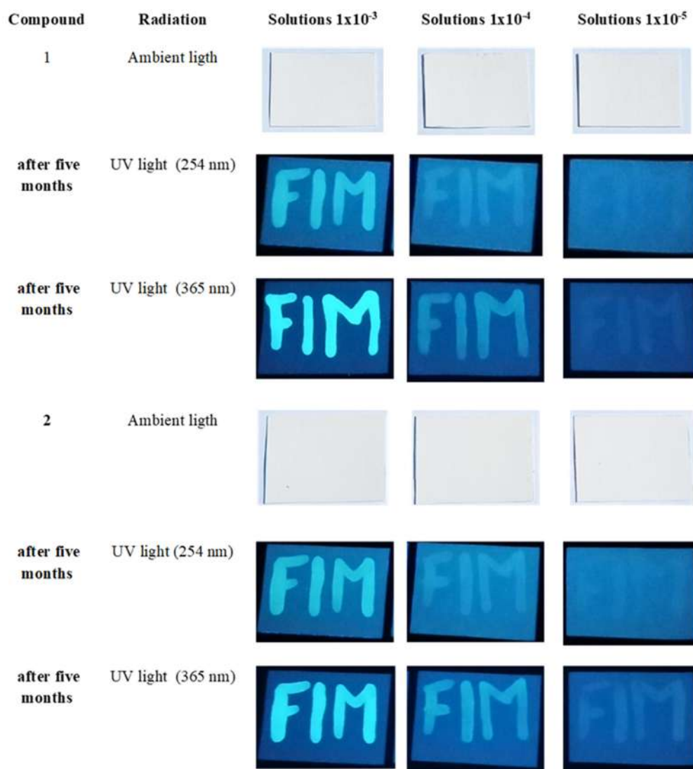
Figure 15. Results of security-ink tests using solutions of complexes 1 and 2 in ethanol with concentrations of 1.0 \times 10^{-3} , 1.0 \times 10^{-4} , and 1.0 \times 10^{-5} M, under ambient light and UV light (365 and 254 nm).
