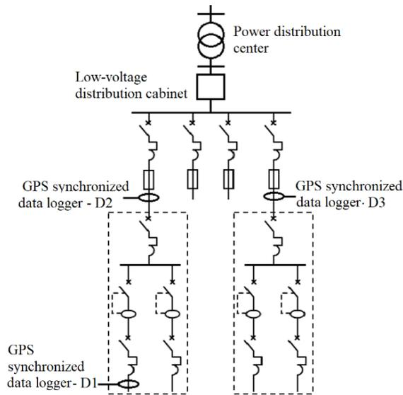
Fig. 7. Setup diagram of the experimental case of study for the monitoring of PQD propagation in an electrical grid.
