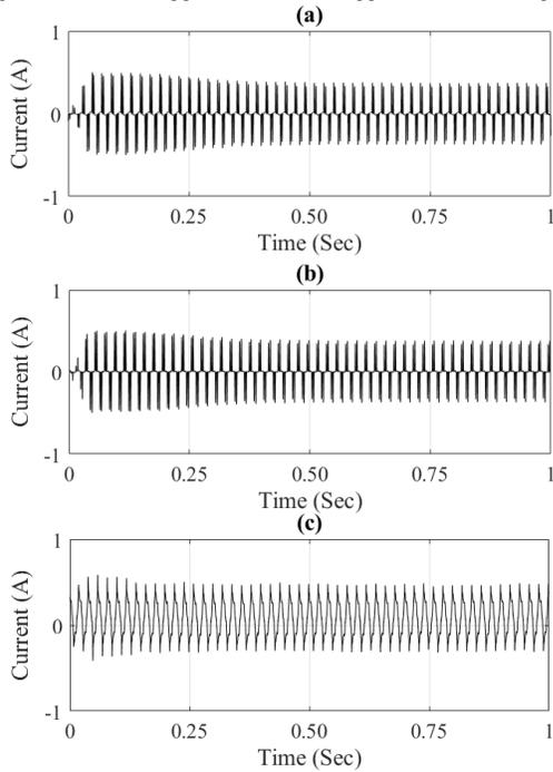
Fig 9. Current signals from GPS synchronized data loggers with PQD propagation. (a) Data logger D1, (b) data logger D2, (c) data logger D3.
