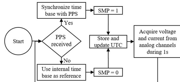
Fig. 1. Block diagram of internal time base synchronization with PPS for each GPS synchronized data logger.
