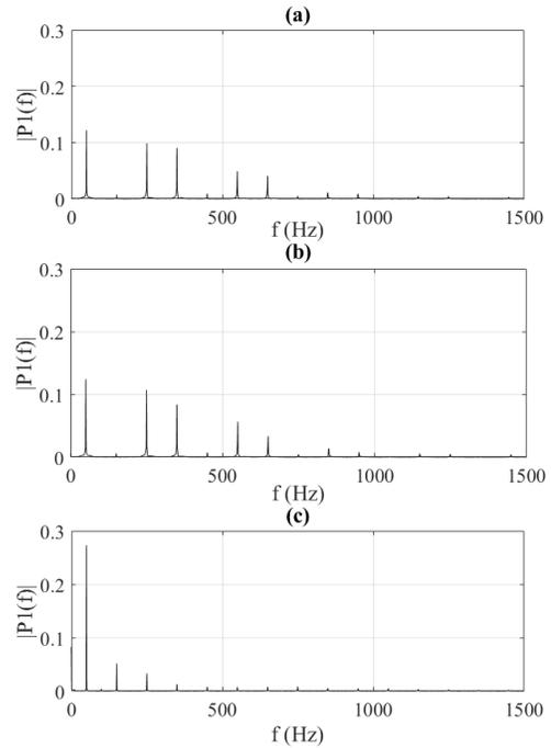
Fig. 10. Frequency spectra of the current signals from GPS synchronized data loggers with PQD propagation. (a) Data logger D1, (b) data logger D2, (c) data logger D3.
