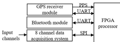
Fig. 3. Block diagram showing the main components of the proprietary GPS synchronized data logger.
