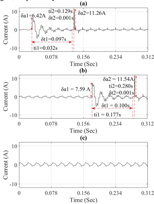
Fig. 8. Current signals from GPS synchronized data loggers with PQD propagation. (a) Data logger D1, (b) data logger D2, (c) data logger D3.
