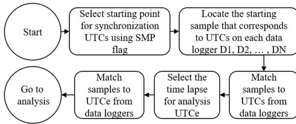
Fig. 2. Procedure to match synchronized signal measured.
