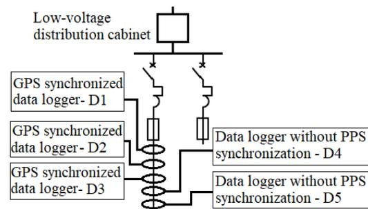
Fig. 5. Setup diagram of the three GPS synchronized data loggers (D1, D2 and D3) and two data loggers without PPS synchronization (D4 and D5) to perform the validation stage.
