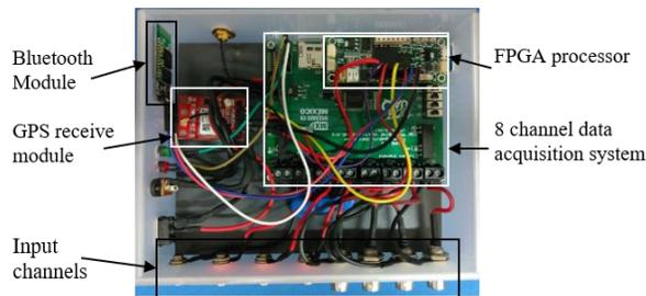
Fig. 4. Photograph showing the main components of the proprietary GPS synchronized data logger.
