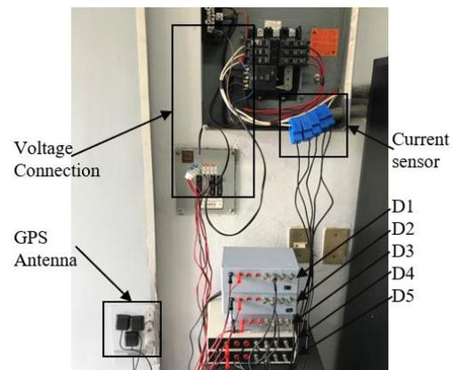
Fig. 6. Hardware connection used to perform the validation stage.
