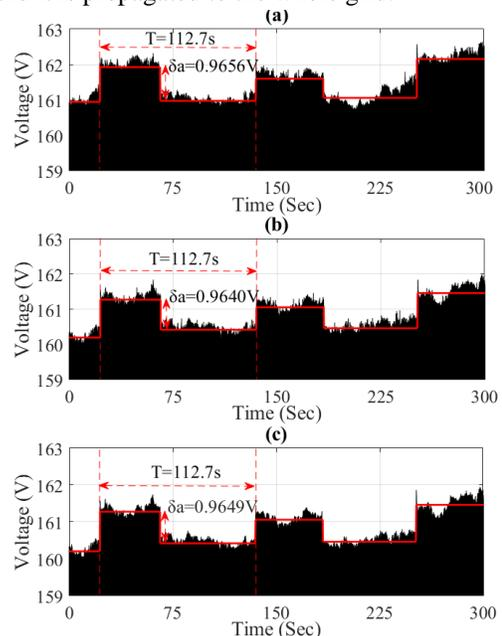
Fig. 11. Zoom at the voltage signals from GPS synchronized data loggers with flicker. (a) Data logger D1, (b) data logger D2, (c) data logger D3.
