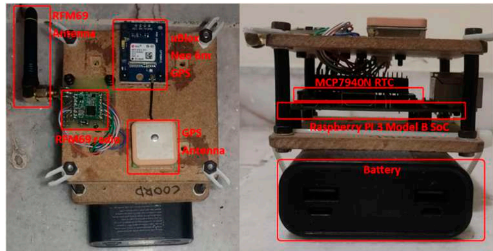
Figure 2. Master node and its components.
