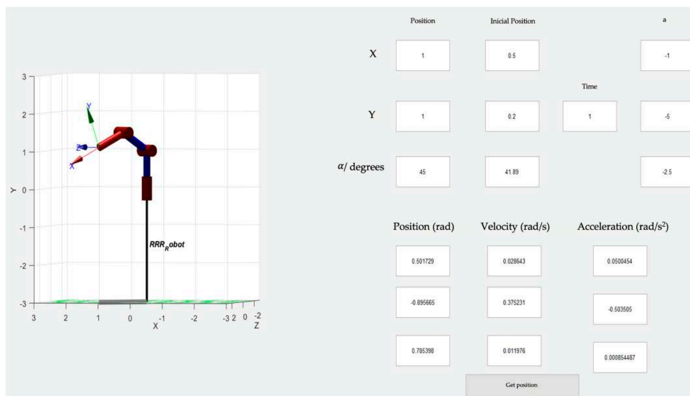
Figure 9. Guide of MATLAB, where the final position (rad), velocity (rad/s) and acceleration (rad/s 2 ) values are shown, and the trajectory is seen with the joint position commands.
