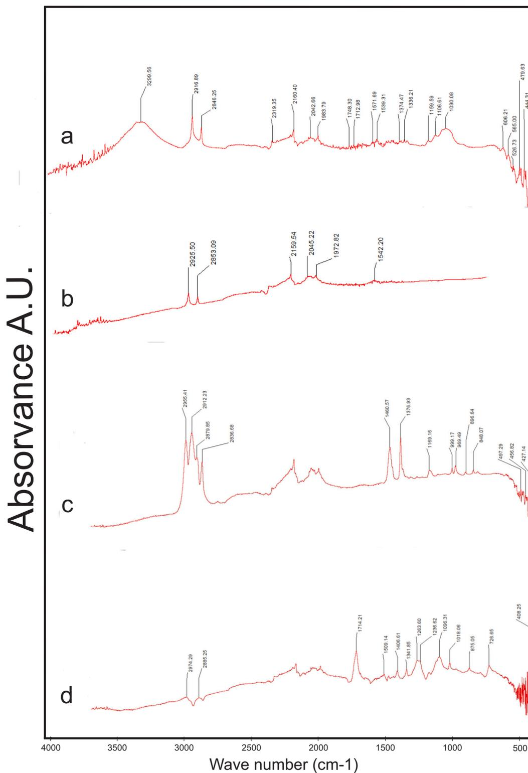
Fig. 5. ATR-FTIR spectra of the plastic particles found in the gastric content of the analysed fish: a) polyamide, b) polyethylene, c) polypropylene, and d) polyacrylic.
