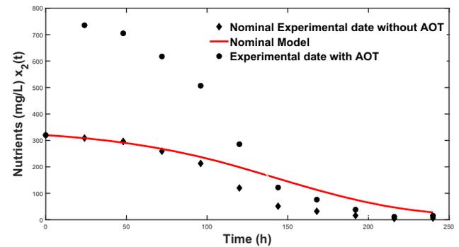
**Figure 4:** Comparison of nutrients with/without AOT recovered substrate feedback and the nominal model.
