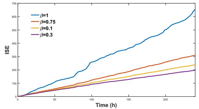
**Figure 9:** Comparison ISE error criteria of the four different controllers with a change in the  $\beta$ .
