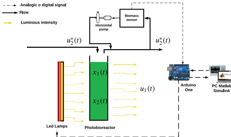
Figure 5: General scheme of lux control and regulation.
