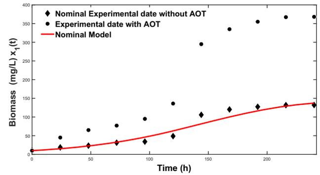
**Figure 3:** Comparison of biomass with/without AOT recovered substrate feedback and the nominal model.
