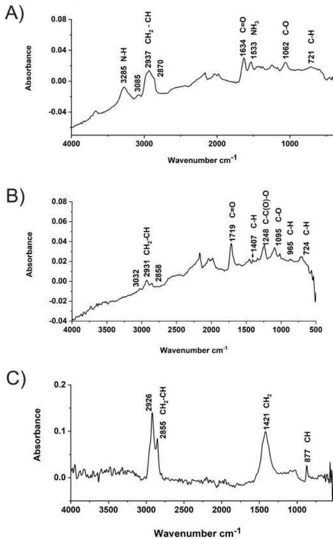
Fig. 3. ATR-FTIR spectra of plastic particles found in the gastric content of Haller's round ray: A) polyamide, B) polyethylene terephthalate, C) polyethylene.
