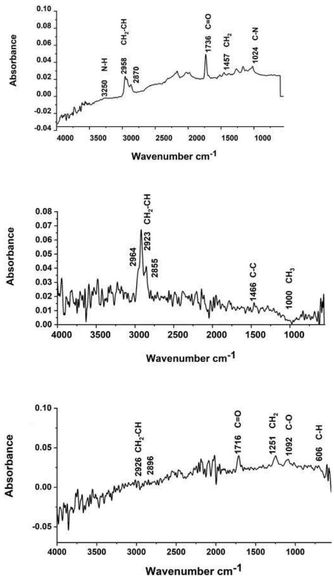
Fig. 4. ATR-FTIR spectra of the plastic particles found in the gastric content of Haller's round ray: A) polyacrylamide, B) polypropylene, C) polyacrylic.
