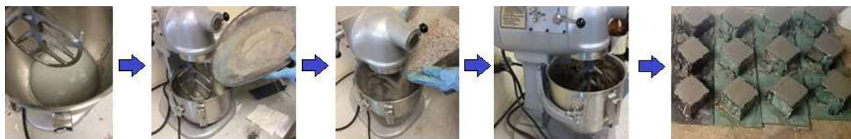
Figure 4. Elaboration of cement mortars modified with PCE, Ss and Ss-PCE.
