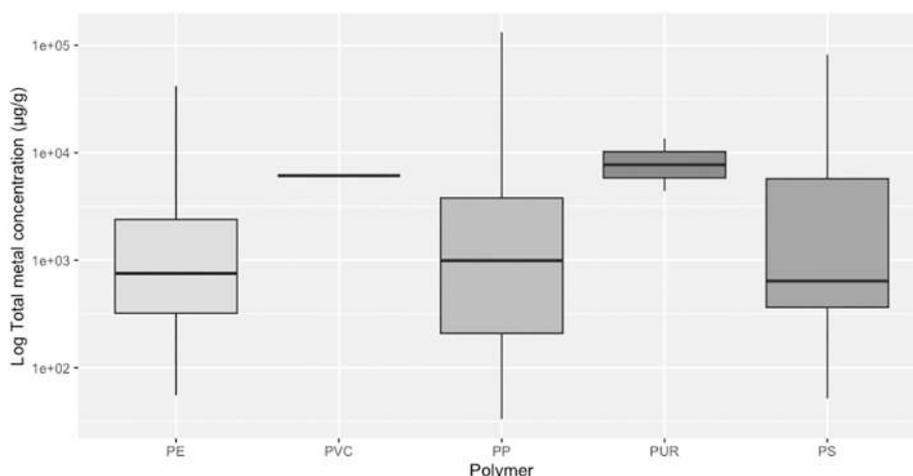
Fig. 7. Box plots showing the metal(oid)s load ( $\mu\text{g/g}$ ) determined in the plastic samples by polymer type.
