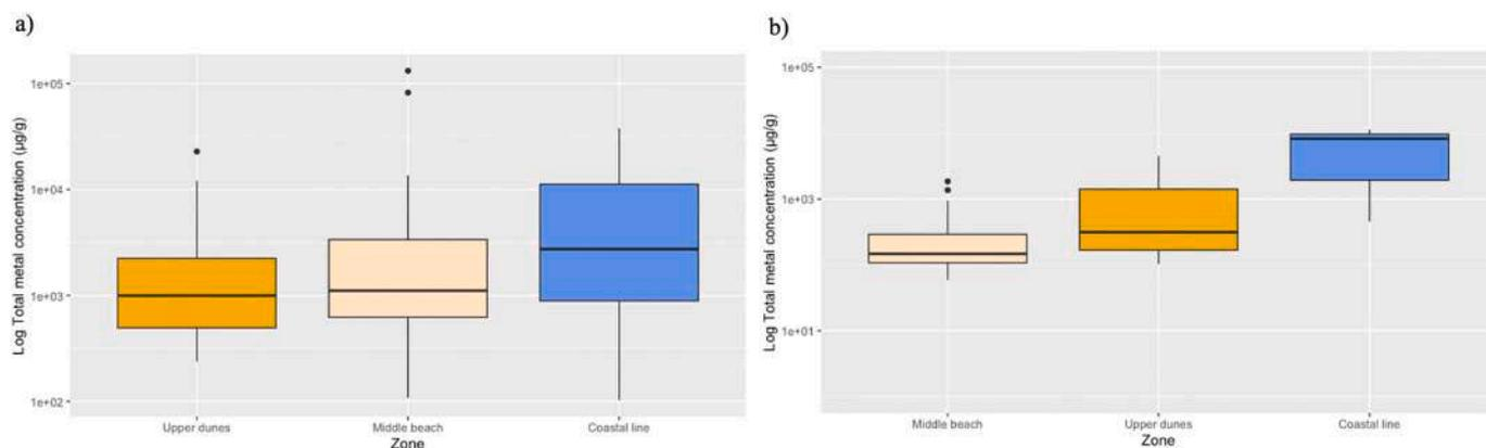
Fig. 6. Box plots representing the Total metal(oid)s content ( $\mu\text{g/g}$ ) determined in all the plastic items by zone for (a) Portman and (b) Calblanque beach.
