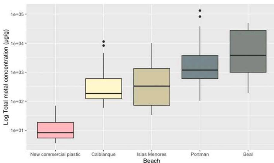
Fig. 4. Box plots representing the metal(oid)s content ( $\mu\text{g/g}$ ) determined in all the plastic items by beach. Levels of metal(oid)s determined in the new commercial plastics were also included here.
