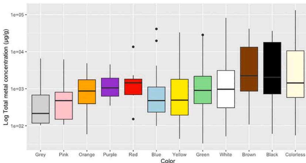
Fig. 8. Box plots illustrating the metal(oid)s concentrations (µg/g) for all the plastic items by color.
