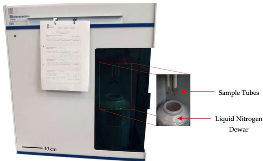
**Figure 2.** Gas adsorption test equipment.
