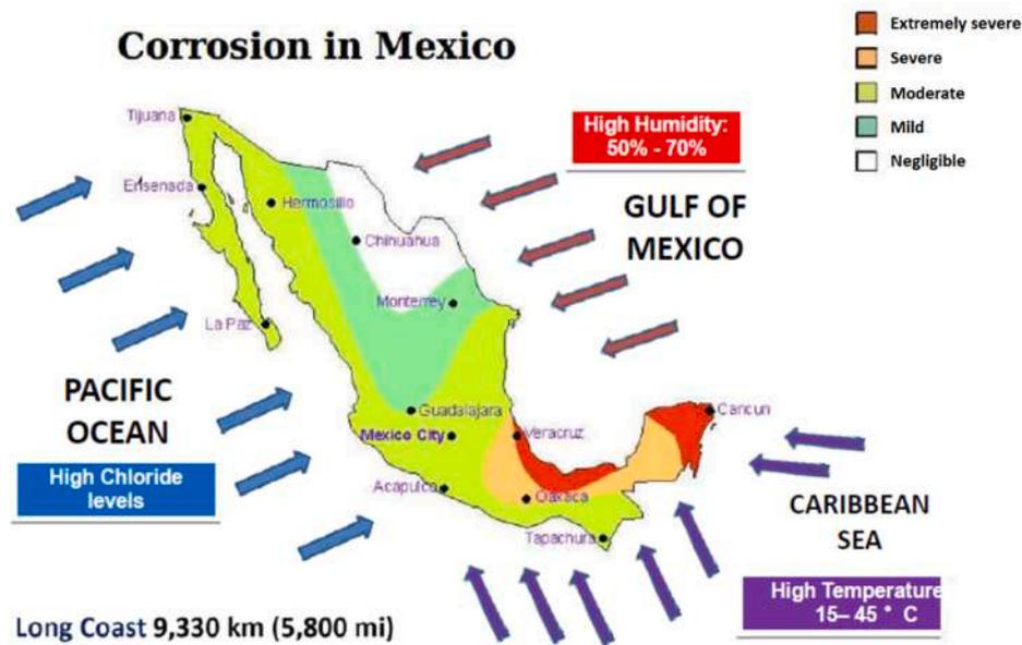
Fig. 1. Main characteristics of the corrosion effects in Mexico [31].
