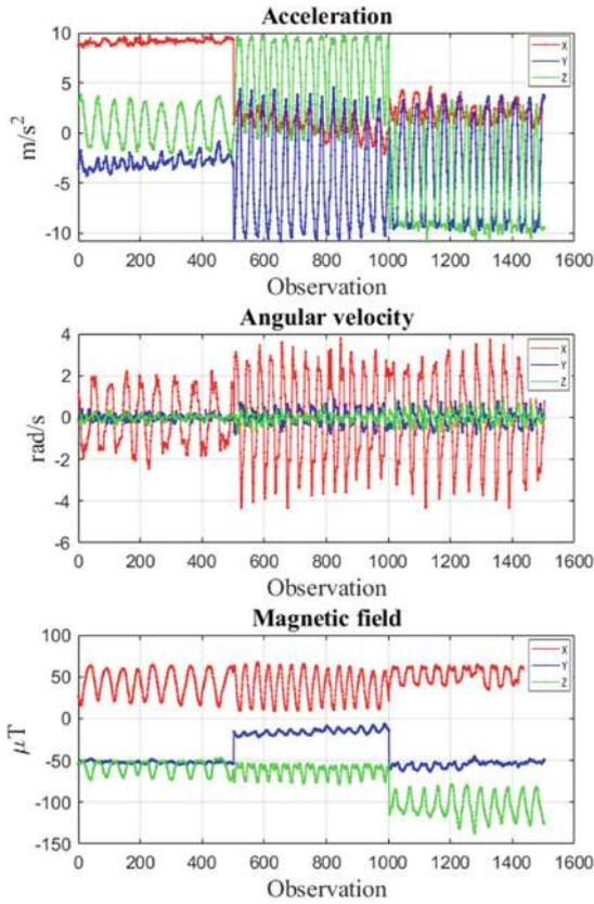
**Fig. 3.** IMU data for flexion-extension of the wrist with a neutral, pronated, and supinated wrist
