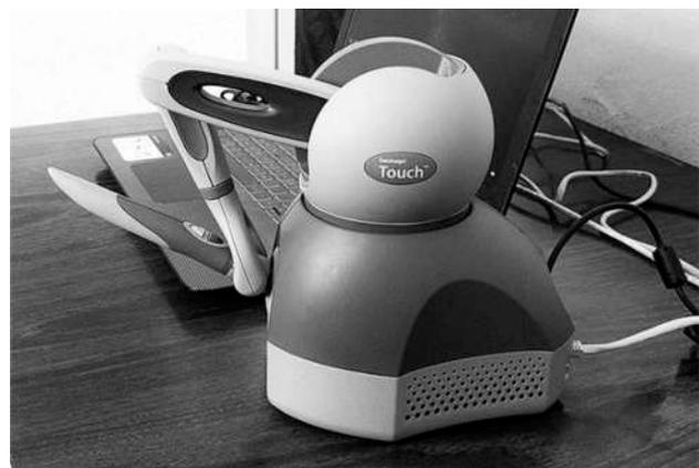
Figure 1. Geomagic® Touch™ haptic interface.
