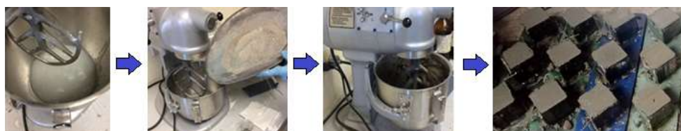
Figure 3. Elaboration of cement pastes modified with PCE, Ss and Ss-PCE.
