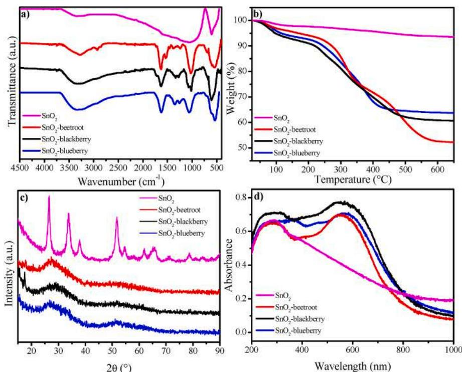
Fig. 1. FTIR spectra (a), thermogravimetric analysis (b), X-ray diffraction patterns (c), and UV–vis absorption spectra (d) for the prepared SnO<sub>2</sub> nanoparticles.
