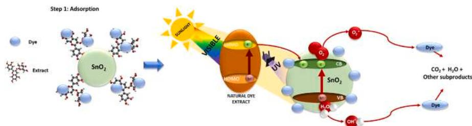
**Fig. 6.** Reaction mechanism of SnO<sub>2</sub> nanoparticles in the photocatalytic degradation of MB.
