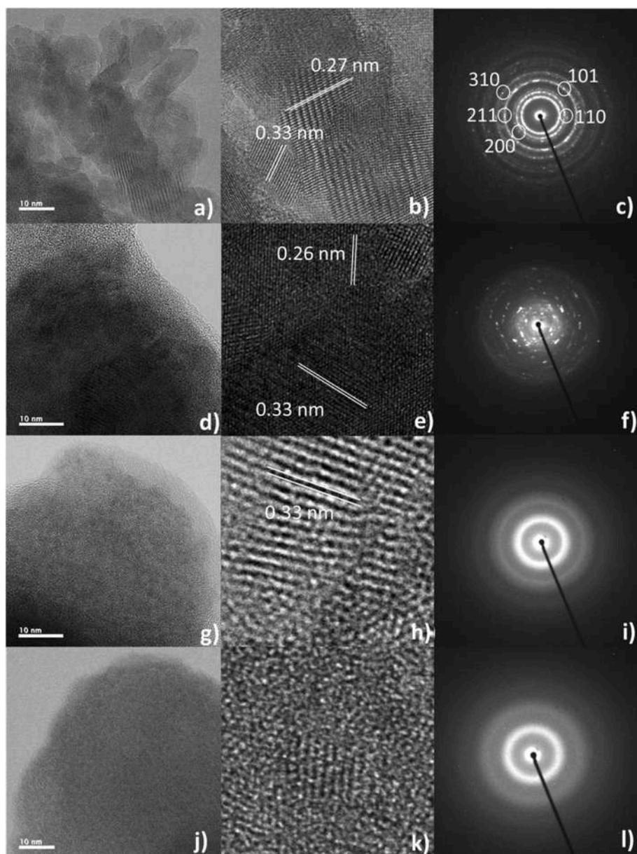
Fig. 4. HRTEM micrographs and SAED patterns of SnO<sub>2</sub> (a–c), SnO<sub>2</sub>-beetroot (d–f) SnO<sub>2</sub>-blackberry (g–i) and SnO<sub>2</sub>-blueberry (j–l).
