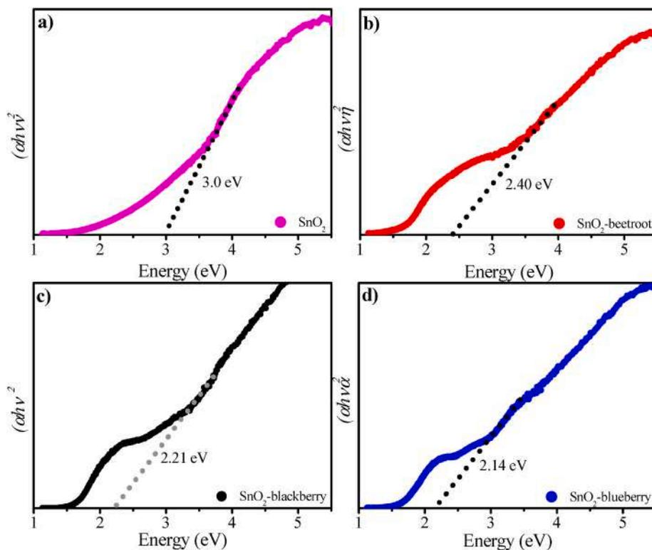
Fig. 2. Tauc plot and band gap values for SnO<sub>2</sub> (a), SnO<sub>2</sub>-beetroot (b), SnO<sub>2</sub>-blackberry (c), and SnO<sub>2</sub>-blueberry (d) samples.
