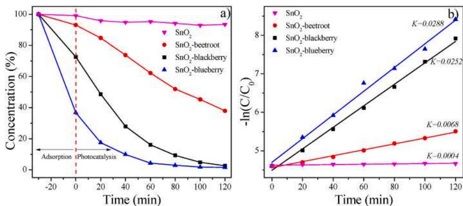
**Fig. 5.** Photocatalytic degradation of methylene blue (MB) under solar irradiation using the SnO<sub>2</sub> nanoparticles (a) and their degradation rate constants (b). (For interpretation of the references to color in this figure legend, the reader is referred to the Web version of this article.)
