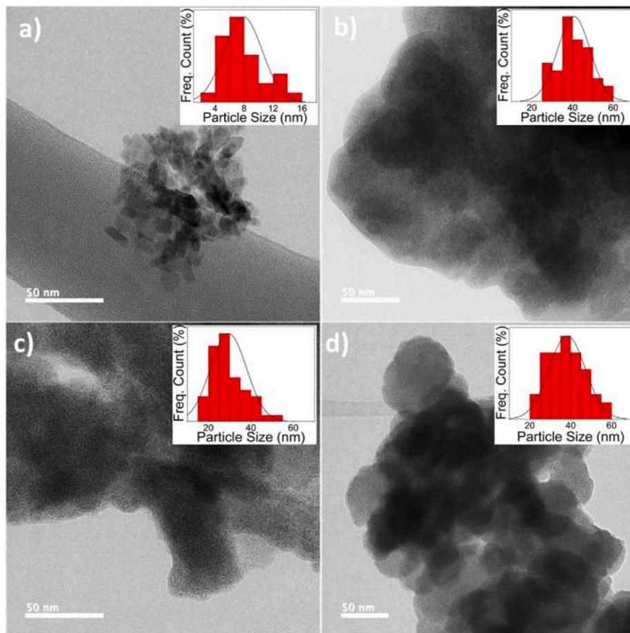
Fig. 3. Particle size distribution and TEM micrographs of SnO<sub>2</sub> (a), SnO<sub>2</sub>-beetroot (b) SnO<sub>2</sub>-blackberry and SnO<sub>2</sub>-blueberry (d).
